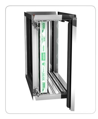
Short depth multistage, convertible, air filter housing ensures that all of the air moving through the system will be treated by the air filters. The Camfil GlidePack MultiTrack 13 is a multi-stage air filter housing with adaptable tracks to apply a variety of prefiltration and final filtration to provide superior indoor air quality for virtually any application. The housing may also be reconfigured in the field for air filtration upgrades or to adapt to the latest air filtration technology.
